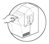
**4.** Press the Clear Button on the front panel to restart the current printer job and to clear the rejected cards counter.
